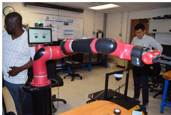
*A team member calibrates the flexible arm which will hold the camera used for non-destructive testing of the tunnel walls.*
