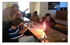
**Heat Transfer** is taught through two experiments involving hot and cold water cups, an aluminum bar, and thermometers. Aligns to Science standards 5.P.3 and 6.P.3.
