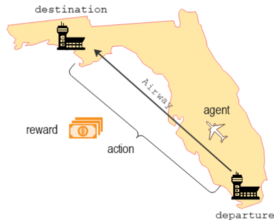
Figure 19. MDP formulation in the L2D. An agent represents an aircraft/pilot. The action in flight dispatch represents assigning the aircraft/pilot to server a particular evacuation flight.
