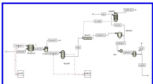
Fig 1. Simulation of pyrolysis of biomass to aromatic H.C
